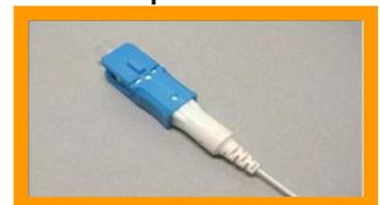
**Rework** - If the connector optical properties are insufficient to use, try re-inserting the fiber.
