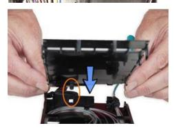
4.4 Lower the cover down to the base. First, lock the rear tabs. Next, align the side and front tabs of the cover with the slots of the base, then press the cover together with the base to lock into place. The module is now complete.
