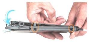
4.5 Insert the module into the desired tray of the ENSPACE patch panel using the white guides. Gently push the module from the rear until it locks into place.
