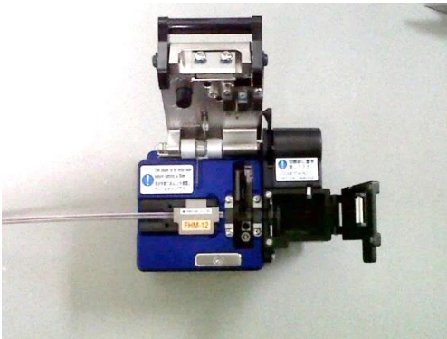
【9】 Remove holder from cleaver and load into left side of splicer
