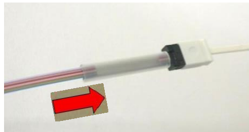
【15】 Remove connector and ribbon from holders and slide sleeve over splice
